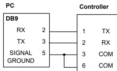
\* Minimum requirements for wiring an RS-232 serial cable to connect to a PC. If you want to connect the controller to a modem, see form #1595, the *SNAP PAC R-Series Controllers User's Guide*, for all eight pin connections.
