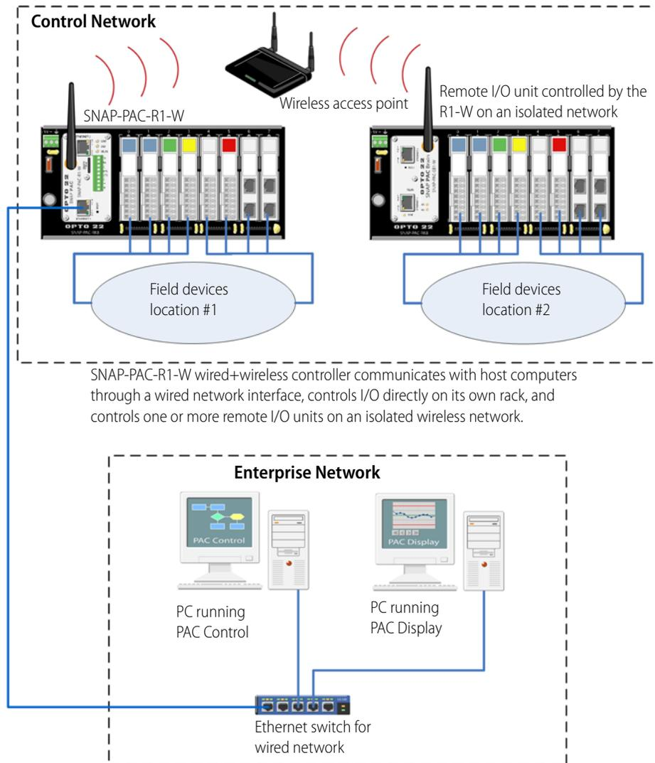
This diagram shows a SNAP PAC Wired+Wireless controller running a PAC Control strategy and controlling one or more remote I/O units via a wireless access point.
