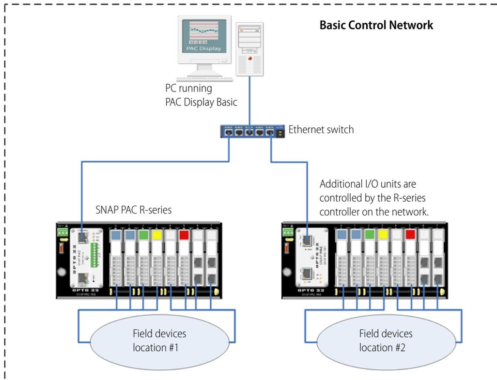
In this diagram, the SNAP PAC R-series controller uses one network interface to communicate with host computers and control I/O. The controller controls I/O on its own rack and on other Ethernet-based I/O units.
