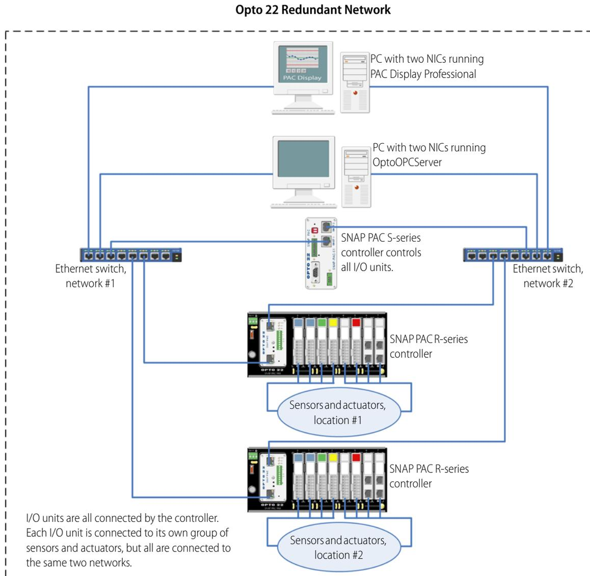
This diagram shows two SNAP PAC R-Series controllers functioning as I/O unit brains connected to two separate Ethernet networks. This configuration addresses the concern that an Ethernet network may fail or need maintenance, leaving the PC running OptoOPCServer and OptoDataLink, the PC running PAC Display, the controller, and the I/O units unable to communicate.
