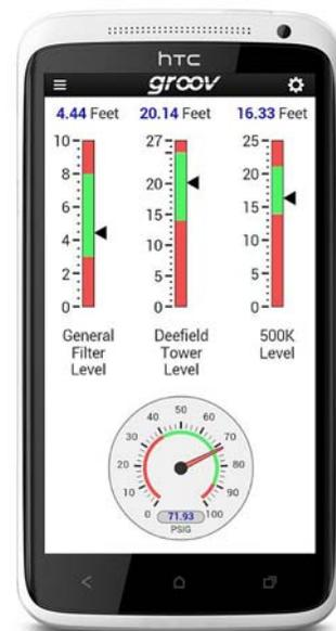
*Tanks levels and pressures are readily available on a smartphone.*
