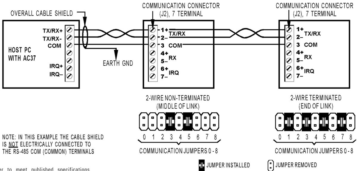
In order to meet published specifications, the RS-485 serial link requires two terminations, one at each physical end of the serial link. **Star configuration is not allowed.** In order to use a star configuration, use Opto 22 Part No. AC38A/B.
