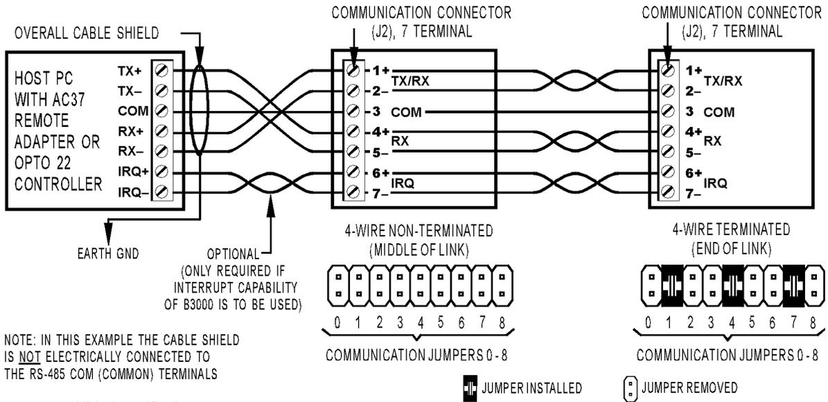
In order to meet published specifications, the RS-485 serial link requires two terminations, one at each physical end of the serial link. **Star configuration is not allowed.** In order to use a star configuration, use Opto 22 Part No. AC30A/B.
